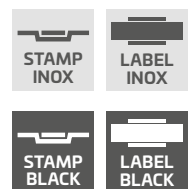
Double-sided embossing width 25 mm with inlay in INOX finish or painted black. The inlay may be placed either on one or on both sides. It is placed in embossing and flush with the leaf (STAMP) or bonded to a flat leaf (LABEL).
