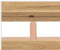
Solid dowel joint
